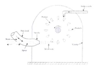
It involves pressure water being converted into kinetic energy. High-speed water from a jet turns a wheel to make it rotate creating kinetic energy which is known as electricity.
