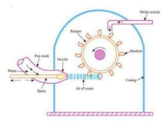
It involves pressure water being converted into kinetic energy. High-speed water from a jet turns a wheel to make it rotate creating kinetic energy which is known as electricity.
